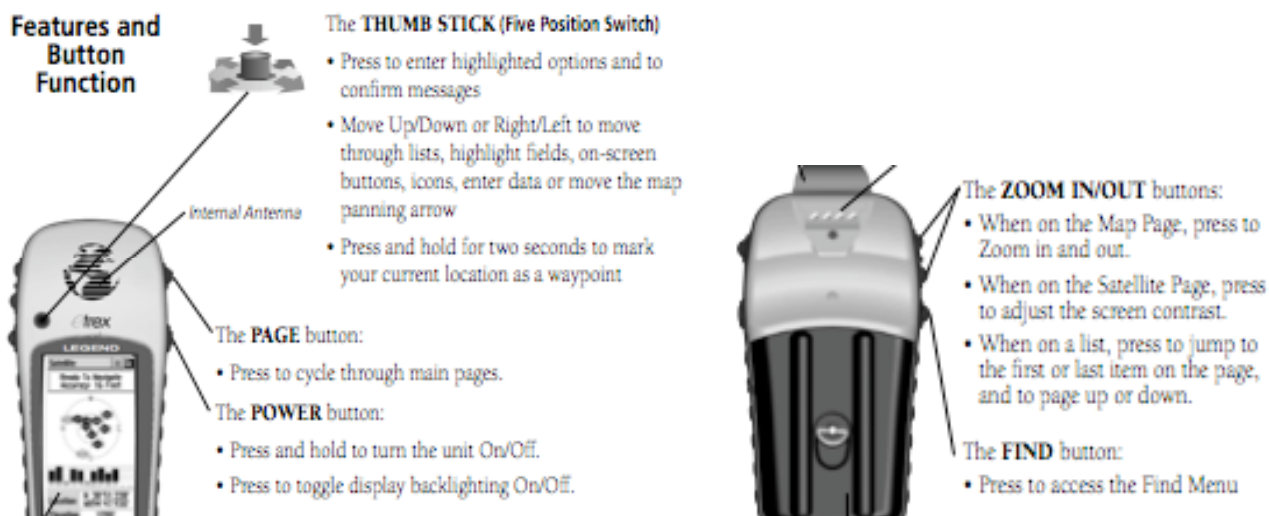
Figure 1: Diagram of buttons on GPS unit and their functions. (Image from Garmin eTrex Legend manual)
